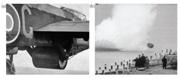
A 4200 kg "bouncing bomb" mounted under a Lancaster B III bombing plane. A mechanical chain runs to the mounting device to induce the backspin necessary for skipping.
