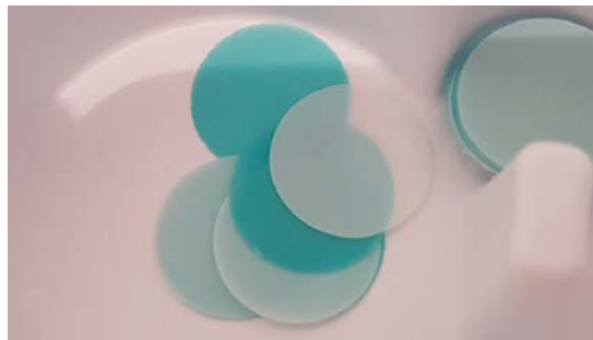
FIGURE 1 – White alumina oxide membranes before coating
