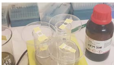
FIGURE 10 – Vapor phase polymerization of PEDOT :Ts
