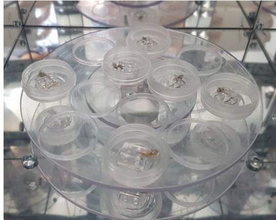
FIGURE 5 – Imaging dishes and their lid in UV curing unit
