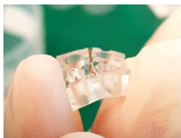
FIGURE 2 – Cut microfluidic chip with membrane inserted
