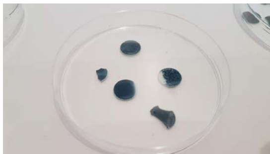
FIGURE 11 – PEDOT :Ts coated membranes
