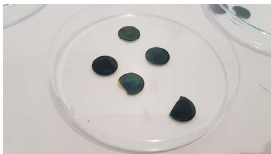
FIGURE 12 – PEDOT :Cl coated membranes
